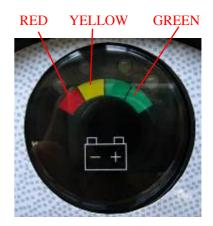
The remaining power suggested by the battery indicator will vary by the actual driving time incurred and how you drive. Repeated starting, stopping, climbing will consume the power more quickly.
