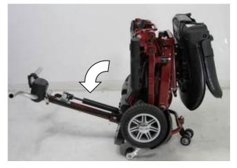
2. Pull the Separate Frame safety Lever to unfolded.
