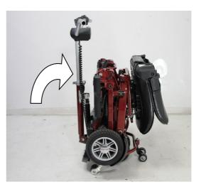
6. Loosen the tiller adjustment lever and fold down the tiller and retighten lever.
