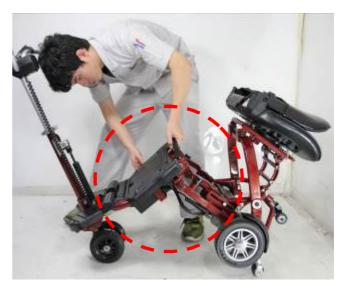
5. push the tiller adjustment knob and fold tiller.
