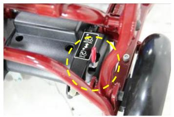
3. Pull the seat adjustment lever swivel seat
