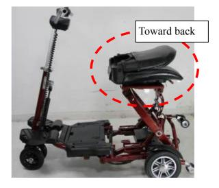
4. pick up the frame separatly with handle bar and fold the rear frame.
