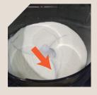
Refill the powder when the powder turnable become visible. This is very important for accurate formula measuring.
