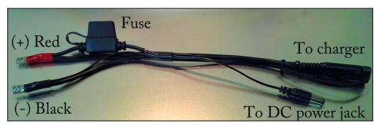
directly from Dry-Flush. Using a fuse rated above 7.5 Amps can cause damage to the electronics or start a fire.
