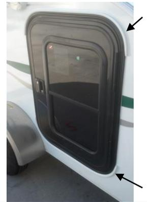
Gutter Rail installed above and below trailer door
