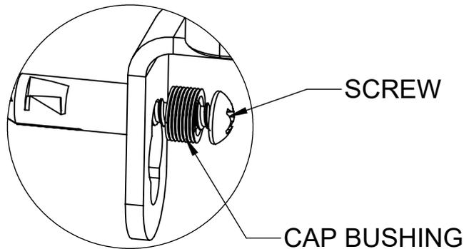
3. Position the shelf unit slipping the angle brackets over the screws and bushings so the screw slips into the upper hole slot. Tighten the 4 screws. When secured to the wall, thread the 4 SCREW CAPS onto the cap bushings.
