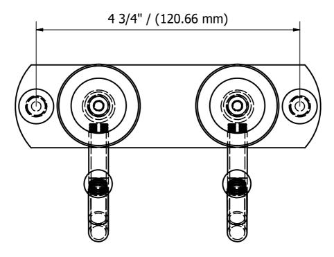
Step2: Attach unit to Mounting Surface.
