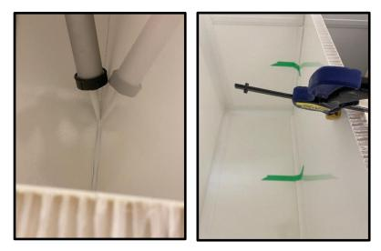
6. To clean up the glued seams we recommend spraying the area with soapy water and then using a plastic squeegee to make the seam look pretty.
