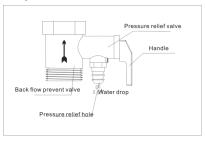
There is a safety valve (pressure relief valve) supplied with the water heater. While the device is heating, expect a few water drops to fall. This is normal as it helps to decrease the pressure in the tank. The back pressure valve ensures that hot water does not flow back into the cold water supply. The safety valve has been preset rated to 7Bar in factory. Do not adjust.
