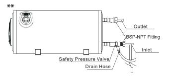
After having installed all water connections, open your water supply and your hot water tap to fill the boiler with water. Once the boiler is completely full, water will run out of the hot water tap. Thanks to its Safety
