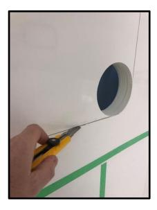
9. Test fit frame from inside of the truck box. Sometimes it is tight and additional cutting may be necessary.
