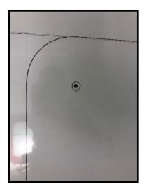
6. Cut each radius corner with hole saw. Drill from inside and outside of truck box body.
