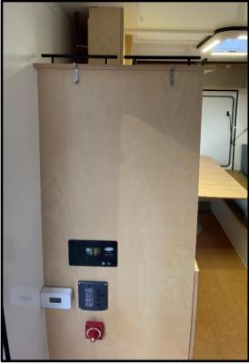
We routed the wires down to the solar controller, switches, and battery disconnect that are mounted on the side of the cabinet. The photos below show the interior of the cabinet and wires going to the battery.
