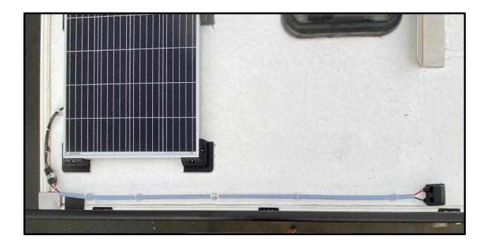
Using a cable entry plate like the one available for purchase off the Expedition Upfitter website the wires are brought down through the roof. The cable entry plate ensures a watertight seal.
