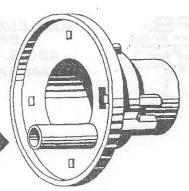
After removal of your old steering wheel, it will be necessary to remove the hom contact plunger and its spring from the plastic hom contact assembly, which should still be on your steering shaft. This horn contact plunger and spring will be replaced in the following manner:
