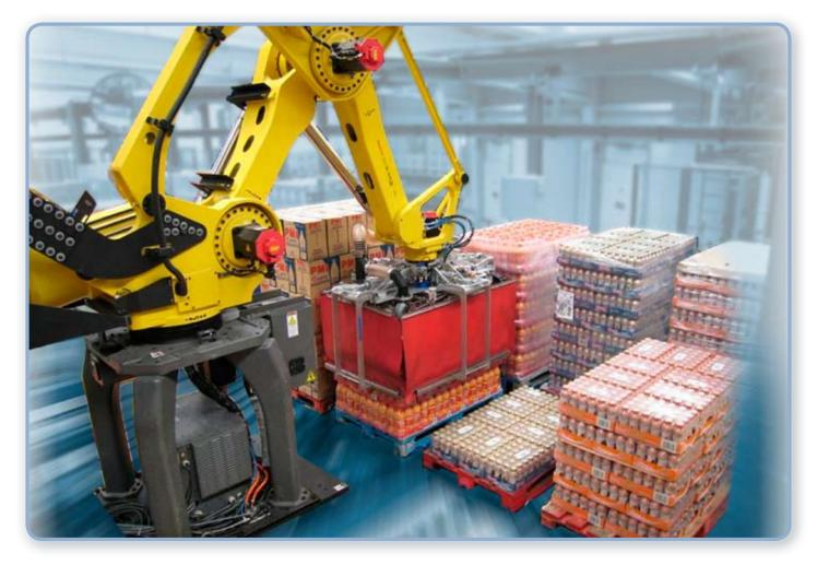
Multi-powered layer handling tool for distribution centres
