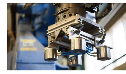
MAP-6, MAP-40 and MAP-180 magnets are especially designed for flat parts that fully cover the magnet's gripping surface. The magnets can also be used with narrow loads and perforated materials, but the gripping force is lower.
