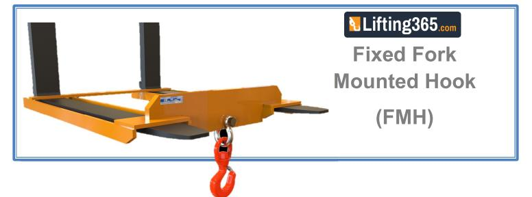
Hugely popular, Fork Mounted Hooks can be fitted to your fork truck quickly and easily; simply, lift the front of the attachment where the hook is located until the attachment is approximately at 45 degrees. The attachment can then be slid on the forks towards the carriage. When the attachment is a far back as possible lower the front down onto the forks and the retaining bar will go up behind the forks and hence the hook is ready for use.
