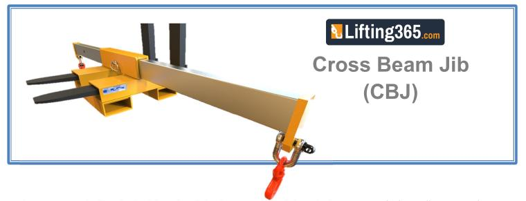
The Cross Beam Jib offers the flexibility tohandle loads via a traditional jib method or via a spreader beam all in one attachment. Simply remove the retaining pin from the beam and slide into the desired position, then replace the pin, ensuring the beam is locked in that position. Then simply drive slowly dorwards until the truck forks are located in the attachment sleeves and simply use the retaining chain to fix the attachment to the forktruck. Then lifting can occur.
