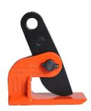
The Tiger CPH clamp is a horizontal lifting clamp intended to be used in pairs, sets of pairs, or in a tripod arrangement for transporting steel plates horizontally. They can be used to lift all types of materials in plate form providing that the plate can withstand the forces imposed on it. These clamps are only suitable for lifting single plates with a surface hardness below 300 Brinell (HB) / 32 Rockwell C (HRC).
