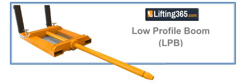
Low Profile Booms (LPB) offer fast and safe transport of rolled/coiled products. To use the boom, raise the carriage until the boom is at the height corresponding to that of the roll/coil. Drive slowly forwards ensuring that the boom is located as far into the core of the load as possible. Lifting can then be effected.
