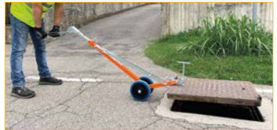
Use 3: mechanical opening with locking clamps.
