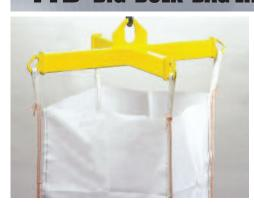
The TTB big bag lifter is designed to lift and transport standard large bulk bags safely and securely. It is manufactured as a 4 point spreader beam in a fixed frame. The construction incorporates 4 hooks with safety latches that allow fast loading and unloading.
