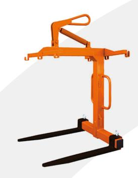
The 1056 has been designed to give flexibility when required to move oversized and normal packs of block and brick s as well as palletised goods around site. This unit is supplied with heavy duty sprung lifting eye allowing automatic levelling of any load being carried. The unit also comes supplied with net hooks allowing the addition of a load safety net
