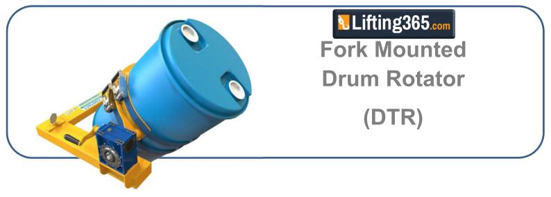
Fork Mounted Drum Rotators are designed for manual rotation of 210 litre drums. The attachment simply slides onto the truck forks, thus allowing 360 degree controlled pouring/rotation via the gearbox. Variations of girdle types are available to suit steel or plastic drums; there is also a model to suit smaller 110 litre drums
