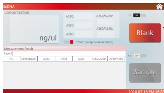
Fig. 3-4 Touch “Blank” button will come out the auto-calibration message at the boot.
