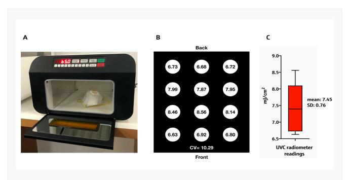
Figure 1. The UVP Crosslinker CL-1000 is a compact, high-intensity, high-uniformity irradiation device. A) Image of the CL-1000 with the front door open and N95 mask placed on the floor of the instrument. B) Diagram depicting the position and intensity of radiometer readings (units mJ/cm²). C) Box whisker summary plot of data from Figure 1B.
