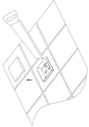
14. Cut extra plastic less than 4mm on the floor.
