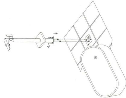
17. Adjust the direction with bath, screw it to the fixed part and close the cover.
