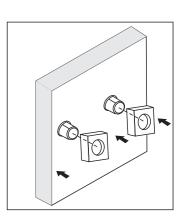
Step 2: Connect the water pipe with the embedded box.
