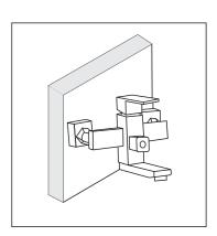
Step 4: After confirm the location, dig out the routes of the pipes. And remove the embedded box and drill the hole. Then use the electric drill to drill white screws into the wall.
