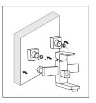
Step 3: Confirm the location of the embedded box and the pipes. Then mark them.
