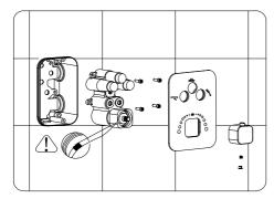
As shown in the figure, install the control valve, and then install the switch handle. Pay attention to the red pen mark. Use the small hexagon wrench included in the package to fix the switch handle clockwise on the valve body of the control valve. The direction of the handle stem is 38  $^\circ$  . position.
