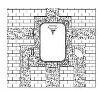
After the installation of the other embedded components of the showeris completed, the embedded box and the pipeline are sealed and fixed with filler.
