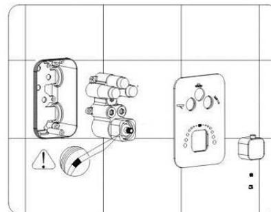
After finish tile wall, remove the clear cover for valve body and then put on face plate as picture.
