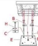
3. Add the screen washer (F). Screw shower hose (G) (not included) to the water inlet on the shower head (E) and then to the water outlet in the ceiling. Install the anchors (A) and fix the mounting bar (B) to ceiling with screws (C). Screw shower bars (D) into the shower head (E) tightly. Attach the shower bar (D) to the mounting bar (B) and fix screws (C) and nut (H) to lock shower bars (D) with mounting bar (B) at the desired height.
