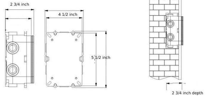
the correct depth for gray box is from 2 1/2 inch to 1 3/4 inch in the finished tile wall.
