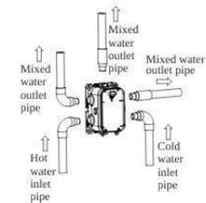
As shown in the figure, the inlet and outlet pipes are embedded. Pay attention to the correct direction of installing the embedded box. Be sure to mark the <sup>TOP</sup> of the baffle upward, and the vertical direction of the embedded box. The lower left interface is connected to the hot water pipe. The interface is connected to the cold water pipe, the upper left interface is connected to the top spray pipe, and the upper right interface is connected to the handheld pipe.
