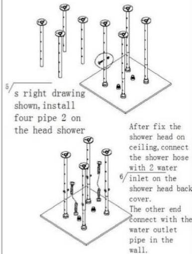
installation steps for 20 inch rain head ( just for flushed on ceiling style)
