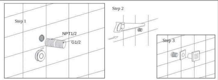
Step 1, Wrap the tooth tube NPT1/2 with teflon tape and screw into the wall
