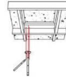
1. Make the fixing positions to ceiling.
