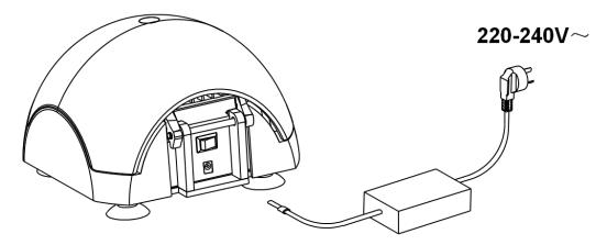
3.3 A safety distance of 30 cm should be observed around the centrifuge during operation. No objects which could cause additional damage in the event of a centrifuge crash should be positioned in this space.
