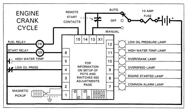
Closure of the Remote Start Contacts while in AUTO initiates the Crank mode. The Fuel Relay and Starter Relay are energized causing the engine to begin cranking. The Crank mode will continue for the duration of the settings of the Crank Cycle Adjust and the Dip Switch, unless Overcrank occurs first. During the Engine Crank Cycle the Low Oil Pressure Switch is ignored. To set Cycle Time and Crank Attempts see adjustments page.
