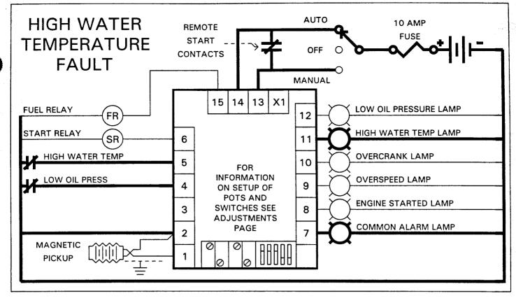
If the High Water Temperature Switch closes the engine will be shut down immediately. System indicates as shown and the LED versions indicate via an LED also. The Engine Switch must be placed in OFF and the engine allowed to cool for reset. The above circuit is grounded fault if you are using positive fault tie your fault switch common to terminal 13.
