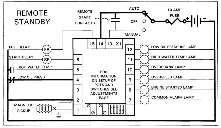
In the Standby mode the Engine Control Switch is in the Auto position as the module monitors the Remote Start Contacts. All that is required for cranking to begin is the closure of the Remote Start Contacts shown connected across terminals 13 and 14.
