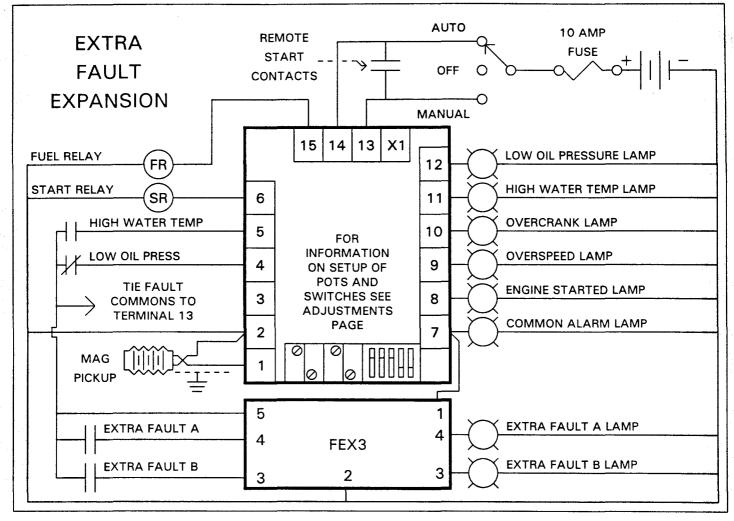
The FEX3 is shown expanding the control to 6 total engine faults. The FEX3 provides both the fault combining signal circuits and the latch circuits. Placing voltage on terminal 7 will place unit in shutdown but it will not latch. See FEX3 literature for more information.
