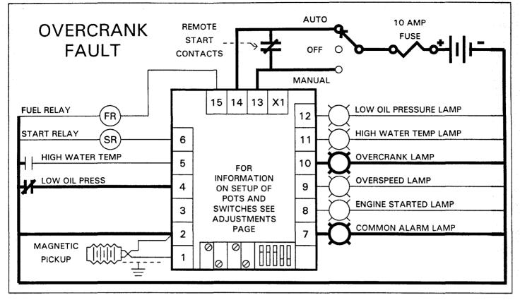
If the engine does not start in the allotted time, as determined by the Crank Cycle Adjust and the Dip Switch settings, the Overcrank Fault occurs. The Fuel and Start relays are turned off and the appropriate signals indicate as shown. The LED versions indicate via an LED also. The Overcrank condition is a latched condition and must be reset via the Engine Control Switch. See Adjustments page for proper settings of adjustments.
