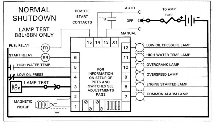
To stop engine place switch in the OFF position and engine will shut down immediately. The Fuel Relay is turned off and the unit draws no power. If the unit is an LED version lamp test may be applied as shown and all LEDS will light. Since the output system is totally independent of the signal system Lamp Test can be actuated at any time with no possibility of backfeed.
