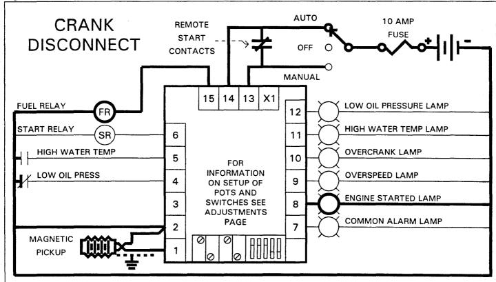
If the internal speed switch detects a speed equal or above the Crank Disconnect Adjustment Setting the starter relay signal turns off, the Low Oil Pressure delay timer is initiated and the appropriate signals indicate as shown. The LED versions indicate via an LED also. This is a latched condition and must be reset by placing the Engine Control Switch in the Off position. The internal speed switch uses the Magnetic Pickup for speed detection.
