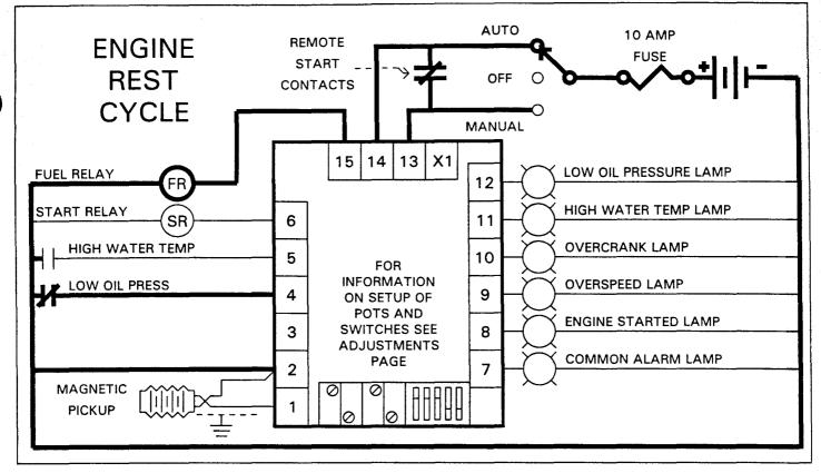
The REST cycle is a pause in the cranking sequence and only applies if Dip Switch 4 on the module is in the Off position. In this mode Fuel is still applied to the engine but the Starter Relay signal is turned off. The cycle continues for the duration of the Cycle time Adjustment Setting. The Low Oil Pressure fault signal input is ignored. To set Cycle Time and Crank Attempts see adjustments page.
