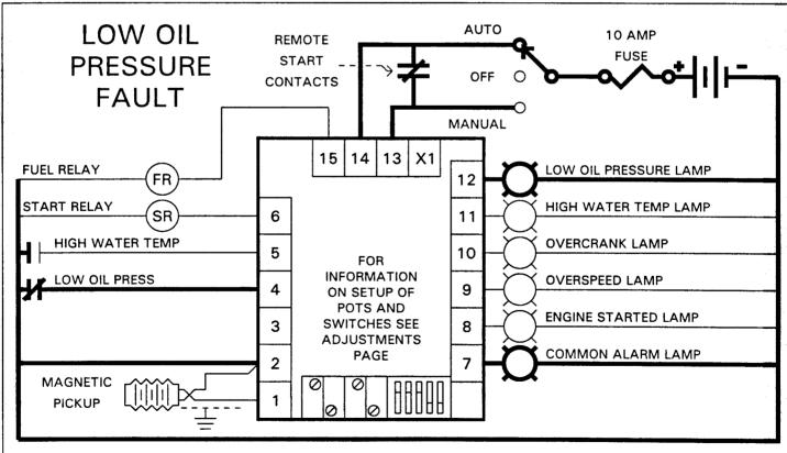
Upon crank termination the Low Oil Pressure time delay begins. After this delay period if the Low Oil Pressure switch closes the engine will shutdown immediately. The Fuel Relay is turned off and the appropriate signals indicate as shown. The LED versions indicate via an LED also. The Engine Switch must be placed in OFF for reset. The above circuit is grounded fault if you are using positive fault tie your fault switch common to terminal 13. See Adjustments page for delay time adjustments.
