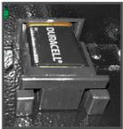
**STEP 3:** Insert a 9V battery into battery compartment & slide battery compartment back into place.
