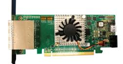
PCIe x16 Gen 4 host interface board with PCIe quad SFF-8644 cable connectors as used in the PCISIG PCI Express External Cable Specification can be configured as x16, two x8, one x8 and two x4 or four x4 cable ports. The cable adapter operates in host or target mode with a DIP switch setting change.
