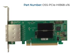
PCIe x16 Gen 3 switch-based host interface board with PCIe quad SFF-8644 cable connectors with ability to be configured as x18, two x8 or four x4 cable ports. The cable adapter operates in host or target mode with a DIP switch setting change.
