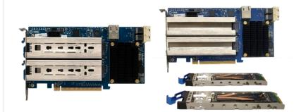
The OSS PCIe 4.0 Dual M.2 Carrier add-in card supports dual PCIe 4.0 hot-swap M.2 drives in removable carriers and dual SFF-8643 connectors for additional NVMe expansion. The hot-swap removable carriers provide high-speed and high-capacity storage at PCIe 4.0 speed for edge applications. Data can be captured at up to 256Gb/s, then securely removed, transported, and hot-swapped into a separate compute node for data processing.
