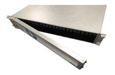
**Step 2: Pull the Drive Tray to mount the storage drive**
