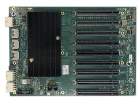
The OSS-BP-581 expansion backplane provides eight PCIe x8 5.0 downstream expansion slots for the latest PCIe add-in cards. Eight downstream slots are single width. The OSS-BP-581 width is optimized to support two backplanes side-by-side in a standard 19" rackmount chassis. The expansion backplane connects back to the host node through the PCIe x16 5.0 upstream slot which can be populated with an OSS-PCIe-HIB732-x16 PCIe x16 5.0 host bus adapter.
