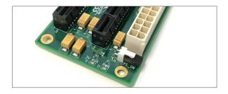
Plug-in the ATX power supply to the "ATX Input Power" connector on the board.
