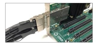
Photos below show the two link cables connected to the target card in the expansion chassis
