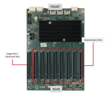
Align the card-edge connector on top of the PCIe slot # 0 (Target slot / Upstream slot).
