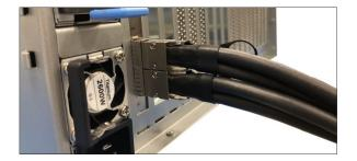
Connect the other end of the cables to the host adapter card.
