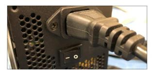
If you are using an external power brick, simply plug-in the power-cord to the brick.
