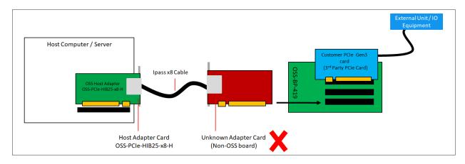
3. Connecting to host computer via onboard / built-in Ipass cable port.
