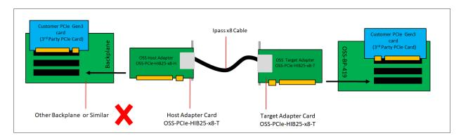
2. Using an unknown target adapter card or other brand of adapter card (made by different vendor).
