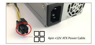
The 4 pin +12 volt cable is polarized so it can only be plugged into the 4 pin board connector correctly. The motherboard connectors and the OSS backplane have the same square and rounded arrangement so the power cable only fits in one way.
