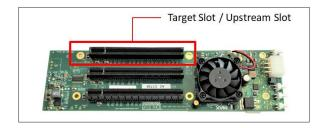
The photo below shows the "Target Card" installed in the Upstream slot.  $\label{eq:card_eq} % \begin{subarray}{ll} \end{subarray} \begin{$
