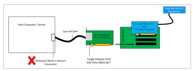
4. Connecting the OSS-419 board to an unknown adapter card and connecting to host computer via onboard Ipass cable port.
