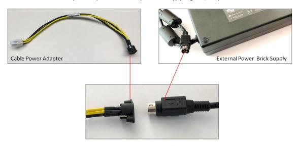
Plug-in the +12V connector to the INPUT connector on the OSS-419 backplane.
