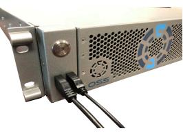
**Step 6: Press the front "Power Button"**Orange LED should come ON immediately upon powering ON the system
