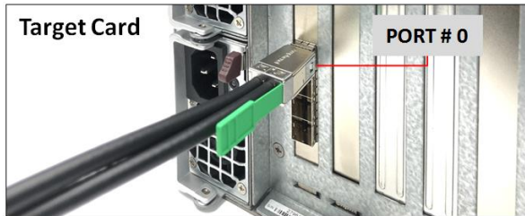
Photo C1: Cable on the Target card is connected PORT #0. The other end of the cable is connected to PORT #3 on the Host card.
