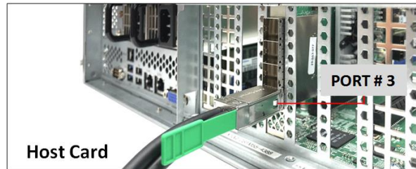
Photo C1: Cable on the Target card is connected PORT #0. The other end of the cable is connected to PORT #3 on the Host card.
