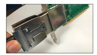
Connect cable to Host adapter card, which is installed in the computer.
