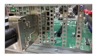
Connect the other end of the cable to the Target card, which is installed in the OSS expansion chassis, see photos below
