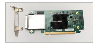
Install the host card in the computer. Plug in the host card in the x16 Gen3 PCle slot. Secure the card.
