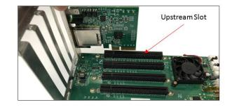
Photos below are different backplanes showing where the location of the Upstream slot.
