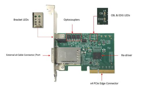
\*The Optocouplers are mounted on the Target card only
