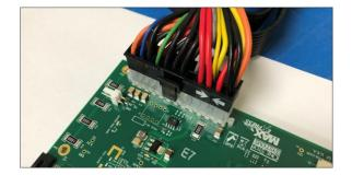
Connect power to the PSU and turn the switch to ON position.
