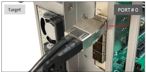
Photo B1: Cable stays connected on the Target card PORT # 0. The other end of the cable is connected on the Host card PORT # 2.
