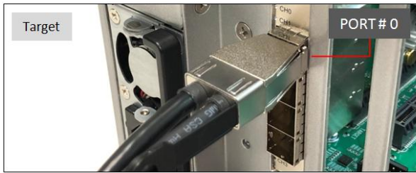
Photo A1: Cable stays connected on the Target card PORT # 0. The other end of the cable is connected on the Host card PORT # 1
