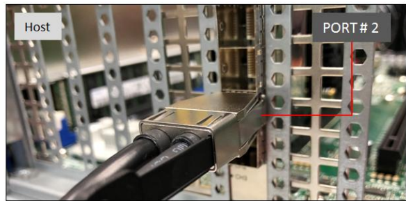
Photo B1: Cable stays connected on the Target card PORT # 0. The other end of the cable is connected on the Host card PORT # 2.
