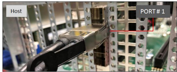
Photo A1: Cable stays connected on the Target card PORT # 0. The other end of the cable is connected on the Host card PORT # 1
