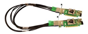
The PCIe x16 Gen 4 expansion kit enables a server to connect to external PCIe Gen 4 expansion slot(s) over cable. The PCIe x16 Gen 4 switch-based cable adapter plugs into a server and cables to a PCIe x16 Gen 4 switch-based target cable adapter. The expansion kit connects over (4) x4, 1 meter SFF-8644 PCIe cables Gen 4.
