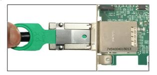
3. Test by pulling back on the connector.
