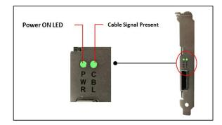
Cable LED indicators are the same for both Host and Target configurations.
