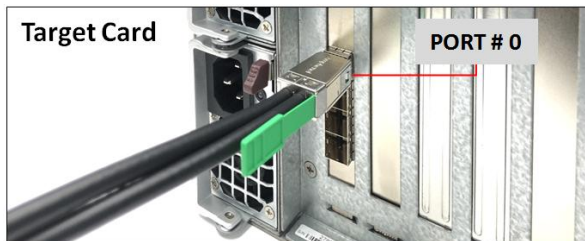
Photo B1: Cable on the Target card is connected to PORT #0. The other end of the cable is connected to PORT #2 on the Host card.
