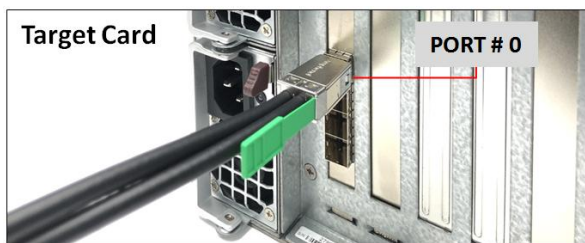
Photo A1: Cable on the Target card is connected to PORT #0. The other end of the cable is connected to PORT #1 on the Host card.
