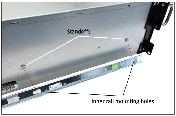
Attach or slip the rail Inner piece on to the chassis standoff, slide and lock.
