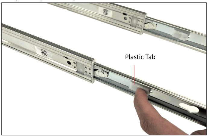
Press and hold the tab, slowly slide the Inner rail out, separating it from Middle rail.
