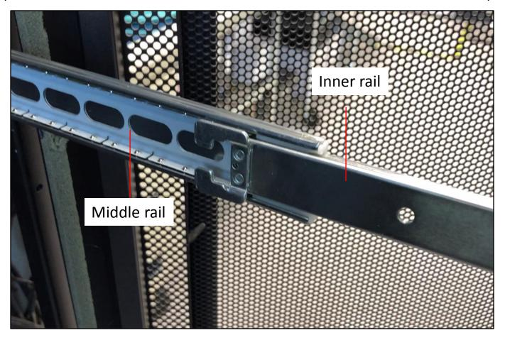
Pull and hold the green plastic tab (both sides) and slowly push the chassis enclosure.
