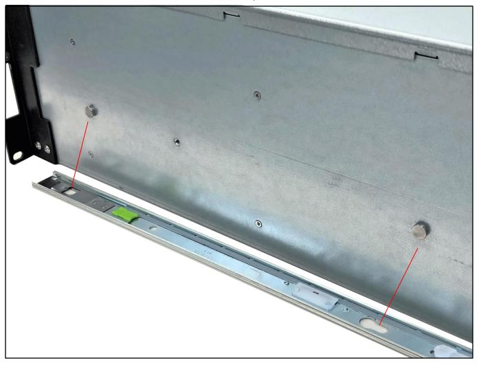
Attach or slip the rail Inner piece on to the chassis standoff, slide and lock.
