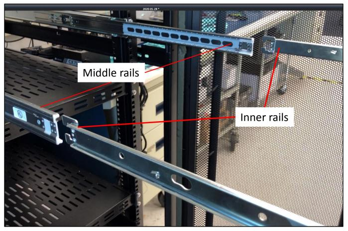
Slowly push the back-end Inner rail from the chassis to the Middle rail until both rails are mated properly.
