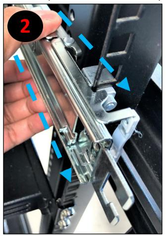
Rear-end rail in "locked position".
