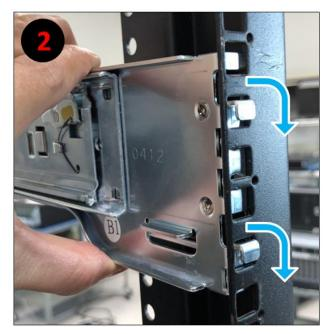
The photo below shows the back-end rail in "locked position".
