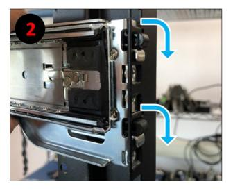
The photo below shows the front-end rail in "locked position".
