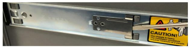
Once you have the flat screw driver inserted, pry out or lift the metal locking latch and push the inner rail outward to dismount.
