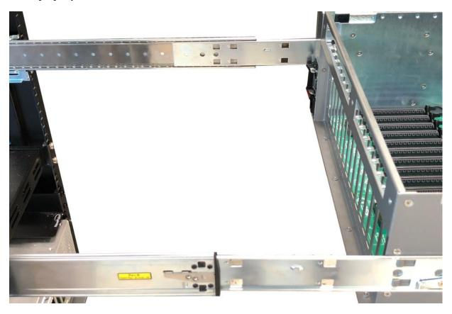
Chassis enclosure  $\/$  expansion unit is now mounted on the rack cabinet.
