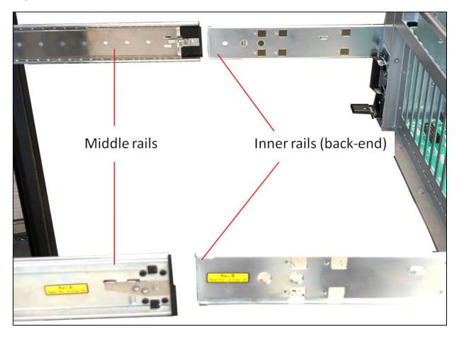
Slowly push the back-end inner rail from the chassis toward the middle rails until both rails are mated properly.
