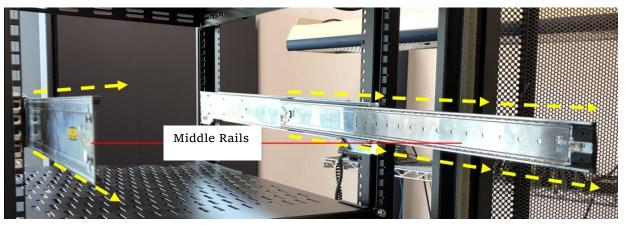
Align the back-end inner rails from the chassis to the middle rails.
