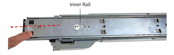
Once the inner rail is fully extended, push down the lever and detach the inner rail from the middle rail.
