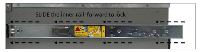
If the rail is unable to slide and lock, you can use a flat screw driver and pry out the metal locking tab while sliding the inner rail towards the front-end. See photos below for the location where to insert the flat screw driver.
