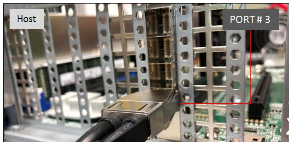
Photo C1: Cable stays connected on the Target card PORT # 0. The other end of the cable is connected on the Host card PORT # 3.
