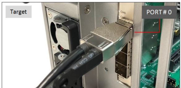
Photo C1: Cable stays connected on the Target card PORT # 0. The other end of the cable is connected on the Host card PORT # 3.
