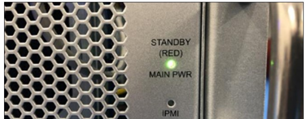
The two front LEDs , the OSS logo will illuminate as blue and the "STANDBY"(MAIN PWR) will come ON as "solid-green".
