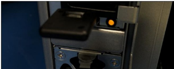
Amber LED: PSU fault or power issue. If Power LED indicator is showing "Amber" in color, it indicates a fault or power issue.
