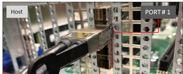
Photo A1: Cable is connected on the Target card PORT # 0. The other end of the cable is connected on the Host card PORT # 1.
