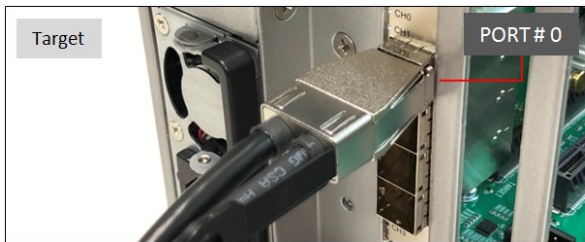
Photo A1: Cable is connected on the Target card PORT # 0. The other end of the cable is connected on the Host card PORT # 1.
