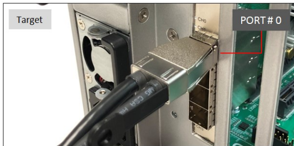
Photo B1: Cable is connected on the Target card PORT # 0. The other end of the cable is connected on the Host card PORT # 2.
