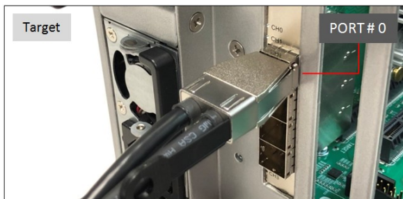
Photo C1: Cable is connected on the Target card PORT # 0. The other end of the cable is connected on the Host card PORT # 3.
