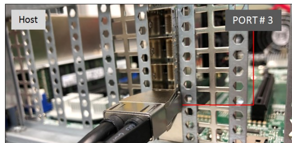
Photo C1: Cable is connected on the Target card PORT # 0. The other end of the cable is connected on the Host card PORT # 3.
