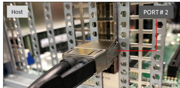
Photo B1: Cable is connected on the Target card PORT # 0. The other end of the cable is connected on the Host card PORT # 2.
